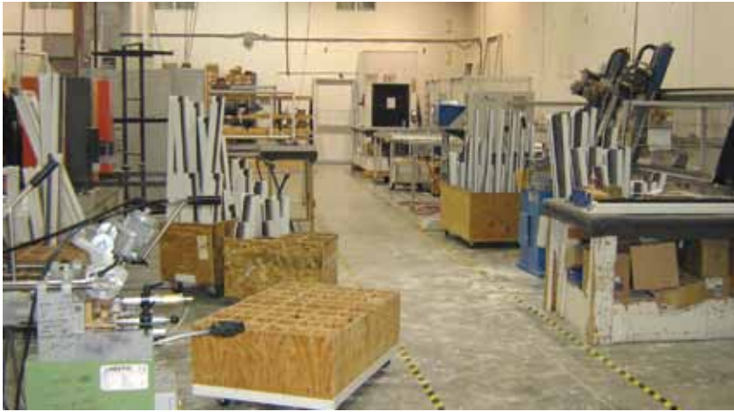
Vinyltek's revamped floor plan puts the machine center, with saw, punches, welder and corner cleaner, in close proximity to reduce wasted product movement.
